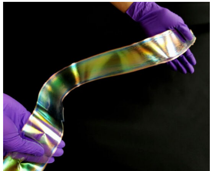
Figura 2 - This gleaming ribbon contains tiny arrangements of eco-friendly cellulose that reflect light in specific ways to give the material its color.
